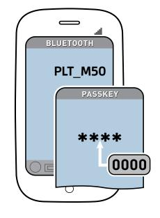
"**Pairing**" is the set-up process of introducing your headset to your phone. Before using your headset for the first time, you must pair it with your Bluetooth-enabled phone.
