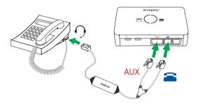
For specific instructions on connecting an electronic hook switch adapter\* to a desk phone, please refer to the cabling documentation supplied with the adapter.
