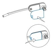
NOTE This product has a replaceable battery. Use only the battery type supplied by Plantronics.
