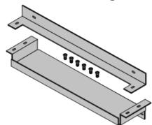
IP500 and IP500v2 control units can be wall mounted. This requires an IP500 Wall Mounting Kit (SAP 700430150) plus additional 4.5mm fixtures and fittings suitable for the wall type. The wall mounting kit includes two brackets, one top and one bottom
